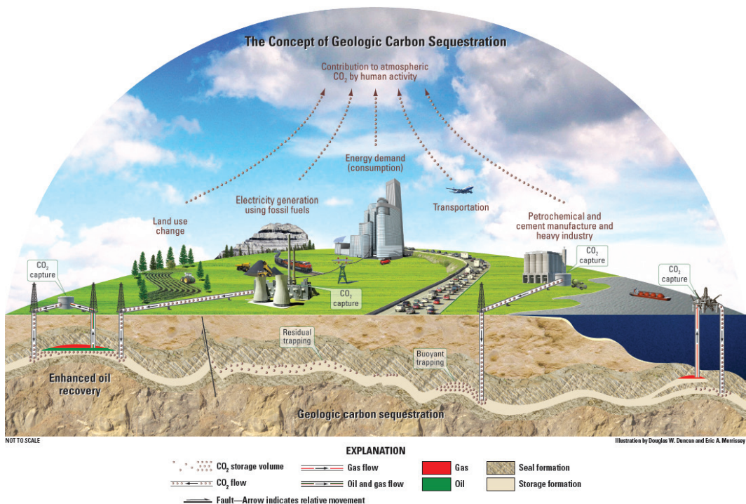
FIGURE 3.14 Illustration of the concept of carbon sequestration. SOURCE: USGS; Duncan and Morrissey (2011).
